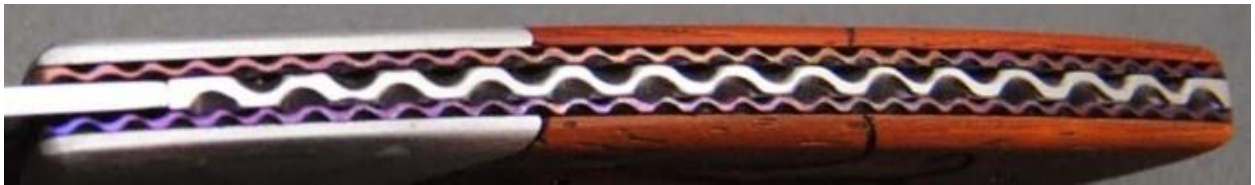
Dots filework on spacer and liners
