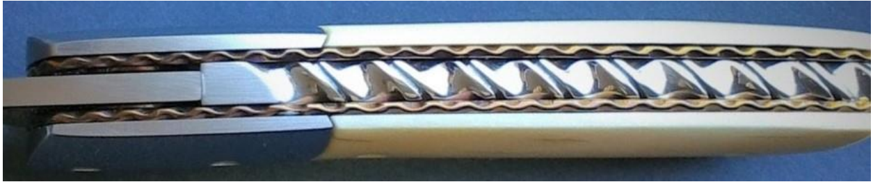
Twisted Ribbon filework on spine and Serpentine filework on liners
