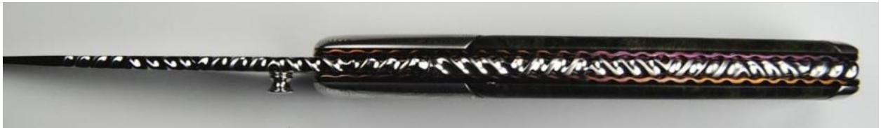
Alternating Twist filework on blade spine and spacer and Serpentine filework on liners
